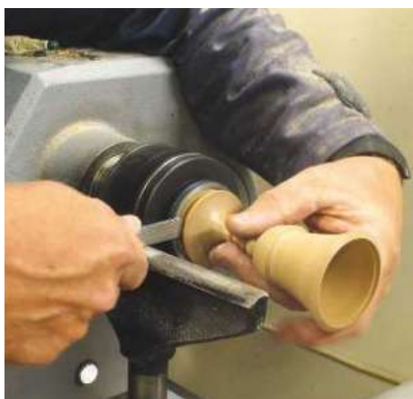
▲ Pic.34 To part off, use the parting tool right handed, lean over the lathe and grip the work with your left hand, making sure that nothing can get caught up in the lathe
